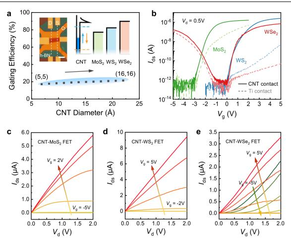
Fig. 4 | General semimetal CNT contacts. a Calculated gating efficiency  $(d\mu_{CNT}/dV_g)$  of armchair CNTs using 20 nm-thick h-BN dielectric. Inset shows the optical image of the as-fabricated device and the band offset between different materials. The white vertical dashed lines represent two CNT electrodes. Scale bar: 5  $\mu$ m. The two horizonal dashed lines represent the gate-tunable work function of
